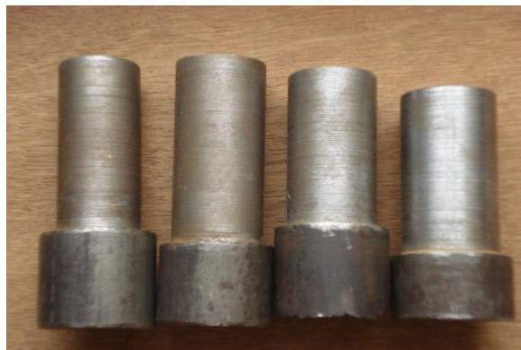
Fig. 5. Mild Steel bars after step turning
