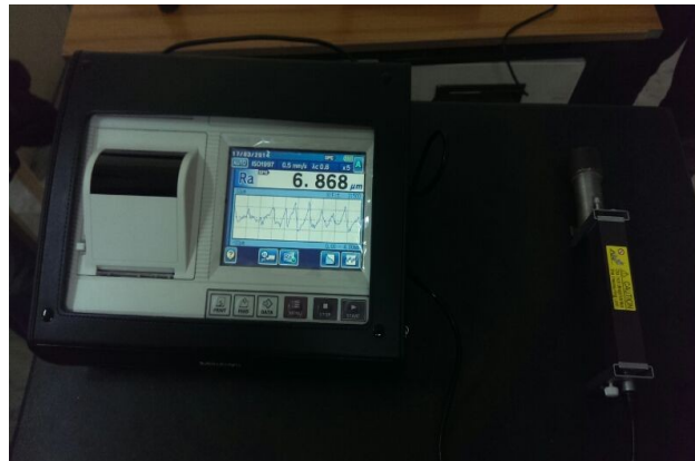
Fig 6: Surface Roughness measurement using Surface Roughness Tester
