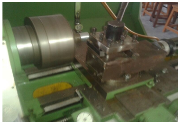
Fig. 4. Step turning operation on lathe
