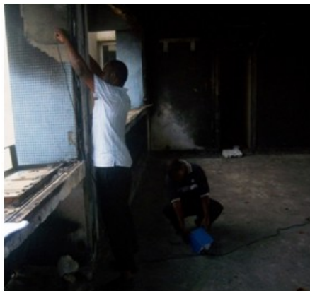
Fig. 6c: UPV test on column
