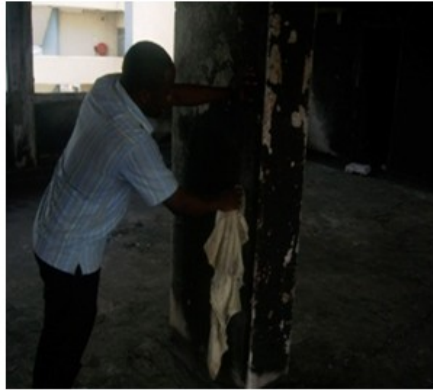
Fig. 6a: Smoothing of the surface to be tested
