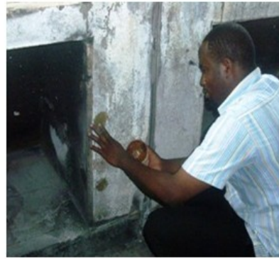
Fig.6b: Grease applied to surface to be tested
