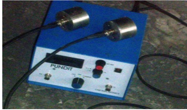
Fig. 4: Pundit Ultrasonic pulse tester Used for the Investigation
