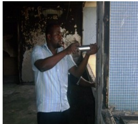
Fig. 6d: RH test on column
