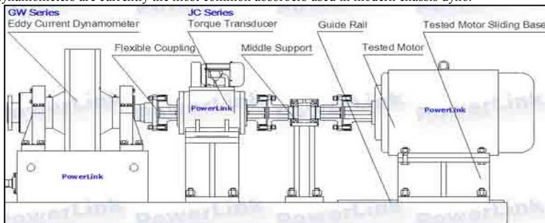
**Fig. 2.2.1** Eddy Current Dynamometer
