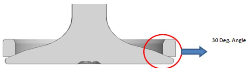
Figure 2.3 Valve & Valve Seat Angle (30°)
