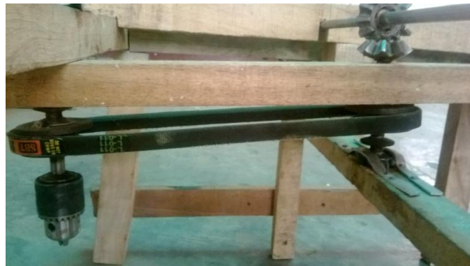
Figure 4: Drilling centre getting drive through bevel gear and belt-pulley arrangement
