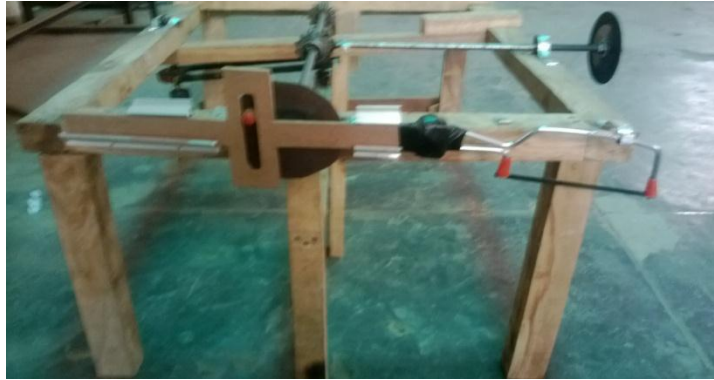
Figure 3: Sawing/ Cutting end using Scotch Yoke Mechanism
