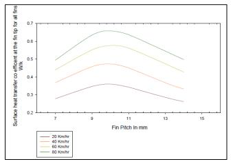
Fig.2.3 Heat dissipated by fins from tip at different velocities [8]
