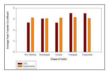
Fig. 2.1 Comparison of heat transfer coefficient (HTC) by CFD and HTC by experiment [5]
