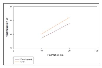
Fig 2.2 Comparison between CFD and experimental results [7]
