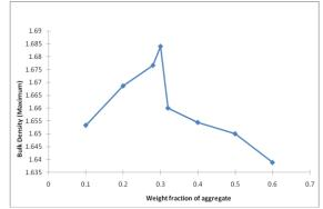
Fig 1: Maximum bulk density for 20mm and 12.5 mm aggregates
