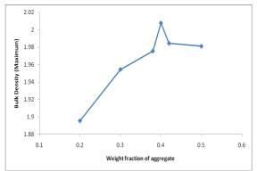
Fig 4: Maximum bulk density for 20 mm, 12.5 mm and fine aggregate
