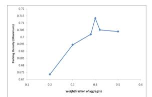
Fig 5: Maximum packing density for 20 mm, 12.5 mm and fine aggregate
