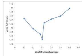
Fig 3: Minimum voids ratio for 20 mm and 12.5 mm aggregates
