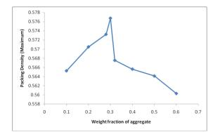
Fig 2: Maximum packing density for 20 mm and 12.5 mm aggregates
