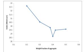
Fig 6: Minimum voids for 20 mm, 12.5 mm and fine aggregate
