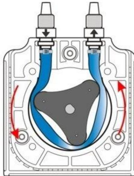
Figure 3.1.1: Basic Shape for rotary peristaltic pump
