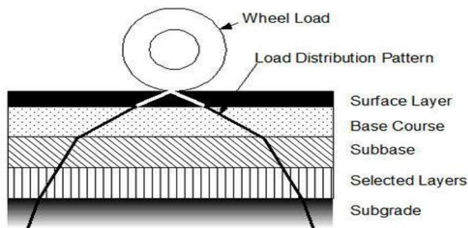
Fig 1. Load distribution of flexible pavement.
