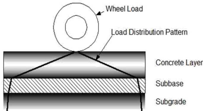
**Fig 2. Load distribution of rigid pavement.**
