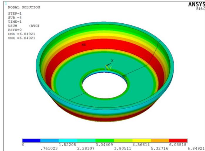
Figure 6: Displacement distribution of component at 3 deg
