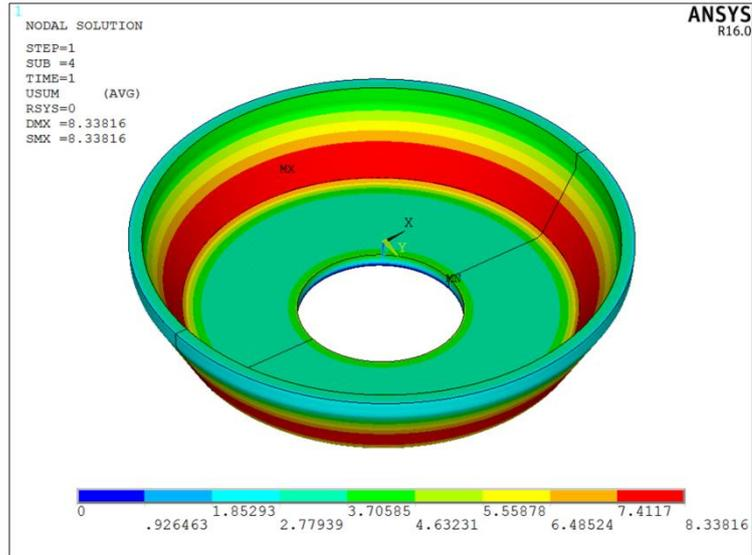
Figure 3: Displacement distribution of component at zero deg
