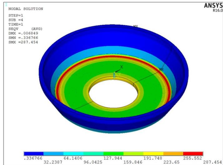
Figure 7: Von-Mises Stress distribution on component at 3 deg.
