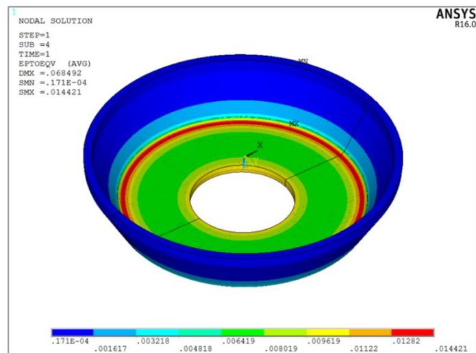
Figure 8: Plastic strain distribution on component at 3 deg.
