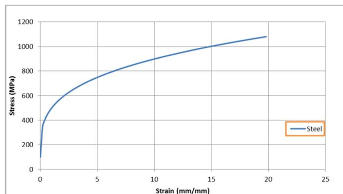
**Figure 2:** Non-linear material properties considered for the analysis
