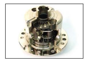
Fig.4 Clutch plate limited slip differential
