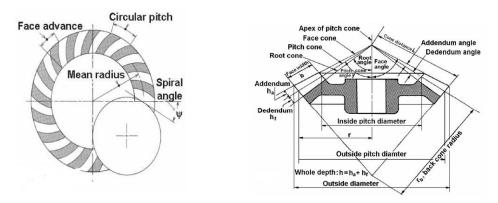
Fig.7 Bevel gear terminology
