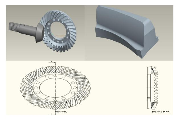
Fig. 8 3-D model of assembly and tooth 2-D view of Crown gear Second National Conference on Recent Developments in Mechanical Engineering M.E.Society's College of Engineering, Pune, India
