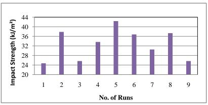
Figure 3 - Effect of fiber parameters in Impact strength.
