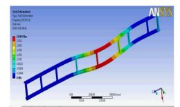
Figure: 3.6 Natural frequency of the existing chassis frame
