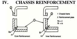
Figure: 4.1 Chassis reinforcement
