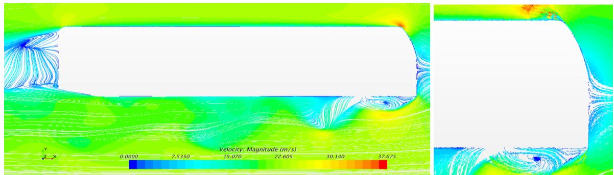
**Figure 2 Path lines on Bus 1**
