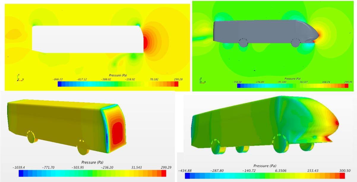
**Figure 1 Velocity and pressure contour for AKN k- $\epsilon$  layer model**
