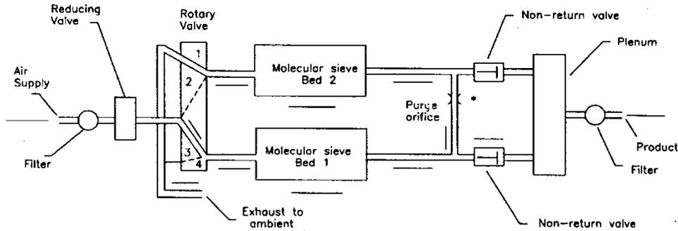
Fig.3 Typical two bed molecular sieve system
