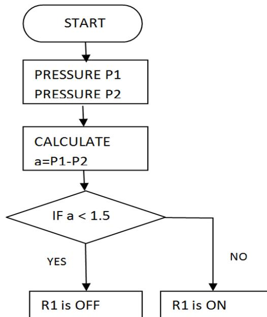
Fig.4 Flowchart of Processor
