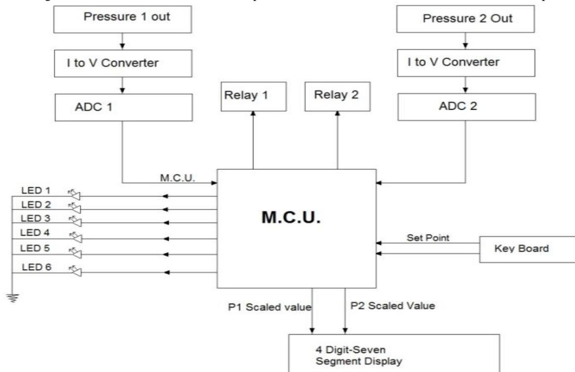
Fig. 6 Hardware Diagram of Microcontroller circuit
