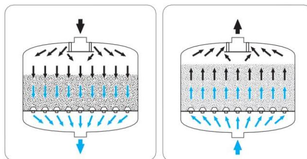
Fig.1 Filtering process
