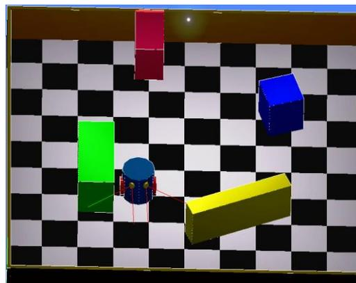
Fig. 2(a) represent the overall configuration of the model (b) show the obstacle detection by mobile robot
