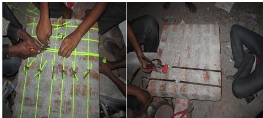
Figure 1- Retrofitting of Specimens and Test Setup
