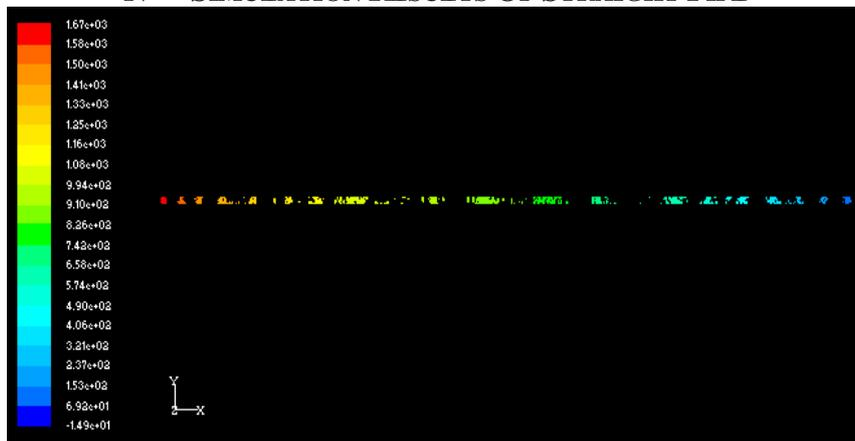
Fig.2. Pressure Display of Bottom Ash at 40% Concentration in 100 meters Straight Pipe
