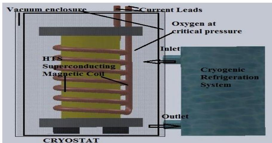
Fig 1: Conceptual 3-D Model of SMES with Oxygen at Critical pressure
