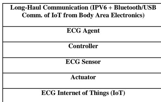
**Fig 1 ECG IoT Stack**
