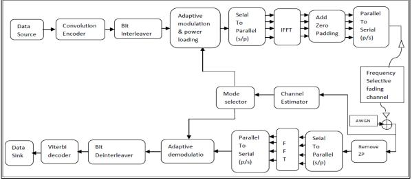
Fig. 1. System model of ABICM with ZP-OFDM
