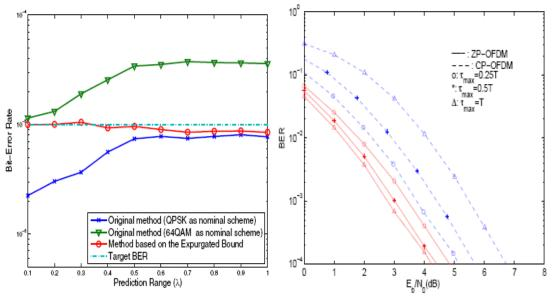
**Fig.5.** BER of ABICM with ZP-OFDM **Fig.6.** BER performance of ABICM-ZP-OFDM w.r.t.  $\tau_{max}$
