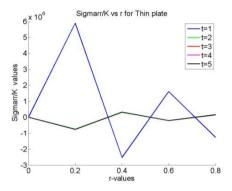
**Fig. 1** Radial stress function  $\frac{\sigma_{\text{rr}}}{K}$  for thin plate(M=0).
