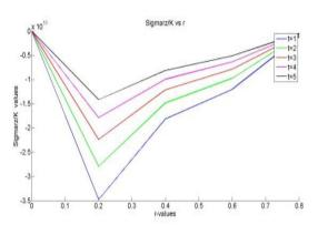
**Fig.8** Stress function  $\frac{\sigma_{rz}}{K}$  for thick plate  $(M \neq 0)$ .
