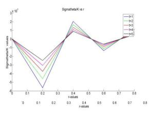
**Fig. 4** Angular stress function  $\frac{\sigma_{\theta\theta}}{K}$  for thick plate  $(M \neq 0)$ .
