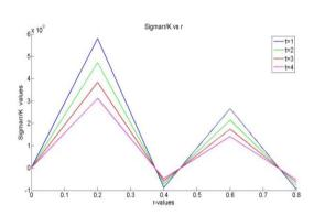
**Fig. 2** Radial stress function  $\frac{\sigma_{rr}}{K}$  for thick plate  $(M \neq 0)$ .
