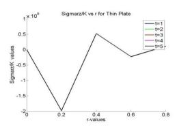
**Fig.7** Stress function  $\frac{\sigma_{rz}}{K}$  for thin plate (M=0).
