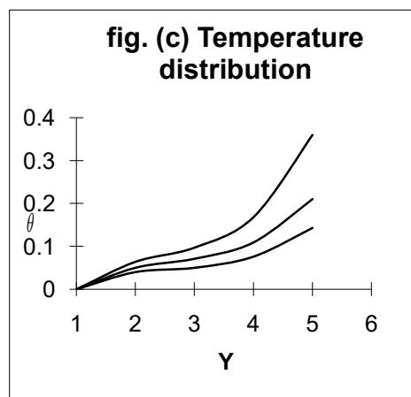
The fig.(c) shows that the rate of heat transfer coefficient at the stationary porous plate. In this case the values of Prandtl number (Pr) are chosen as 0.5 approximately, which represents air and water at  $15^0 C$ . Here it is found that the rate of heat transfer is much lower in the case of water than in air.
