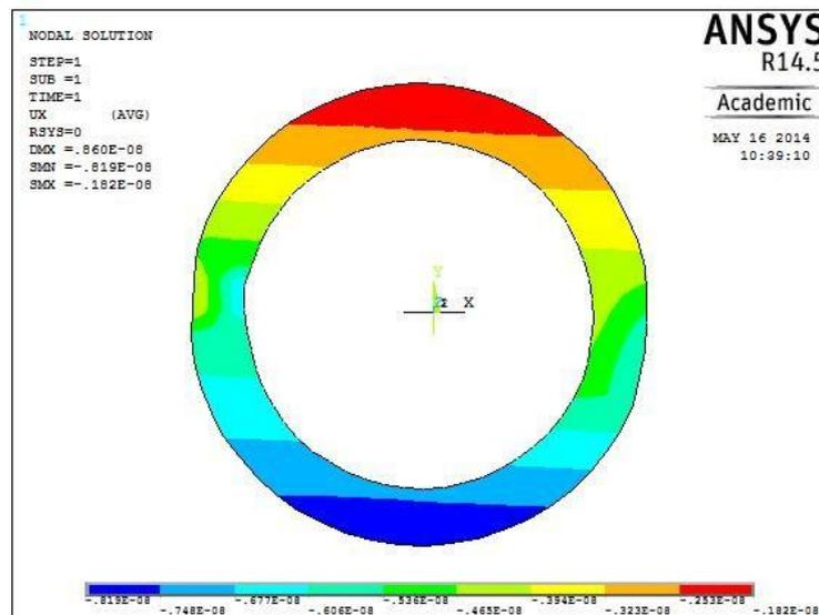
Figure 8: Deformation of a PZT ceramic subjected to an electric field
