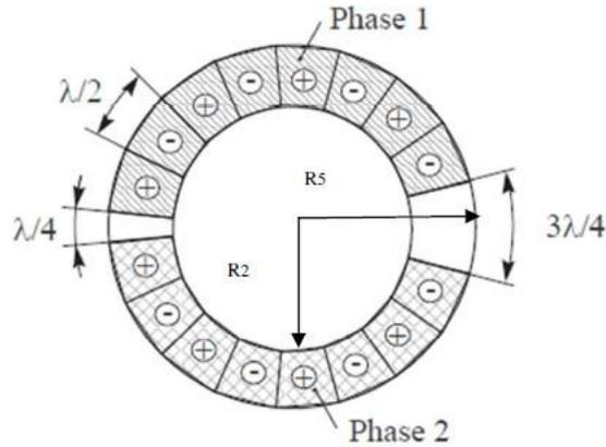
Figure 6: sectorization of a piezoelectric ring used in a progressive wave motor
