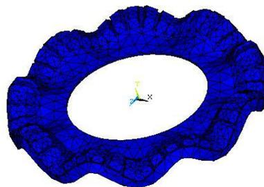
**Figure 5:** The first mode of the stator
