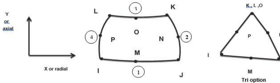
Figure 7: geometry of PLANE223
