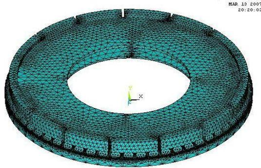
**Figure 3:** Meshing the stator and rotor
