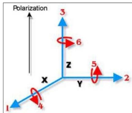
Figure 1: Repere associated with stress and strain vectors
