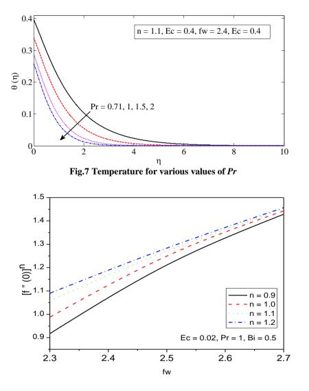
Fig.8 skin-friction for different values of  $f_w$  and n.
