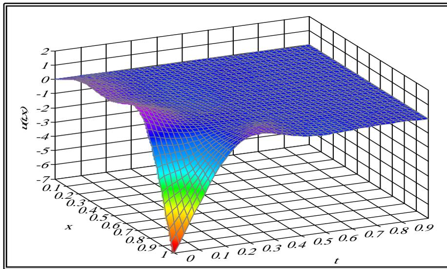
Fig.(1) Closed-loop response with controller for the heat equation (19).
