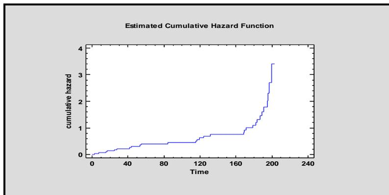
**Figure (3):** Cumulative hazard function vs time for machine no(1)
