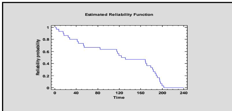
**Figure (2):** Reliability function vs time for machine no(1)
