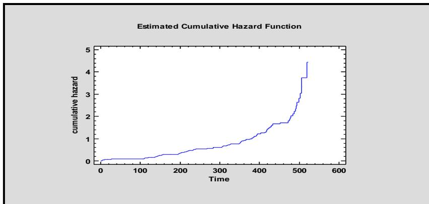
**Figure (7):** hazard function vs time for machine no(4)
