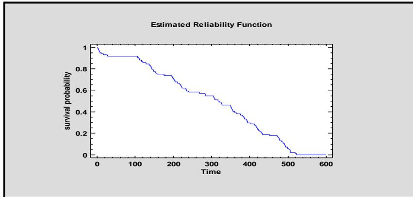
**Figure (6):** Reliability function vs time for machine no(4)
