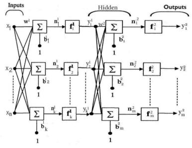
Figure 3. Three layer feedforward neural networks
