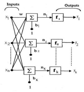
Figure 2. Single layer feedforward neural networks
