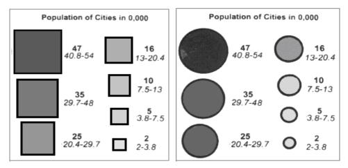
Figure 6. Prototypes of improved legend design and arrangement in proportional circle and square symbolised maps. Bold figures denote class geometric means used as radii for standard symbols in legends. Figures in italics show the class limits.
