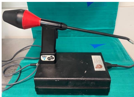
Figure 1: Infrared equipment (generator and gun)
