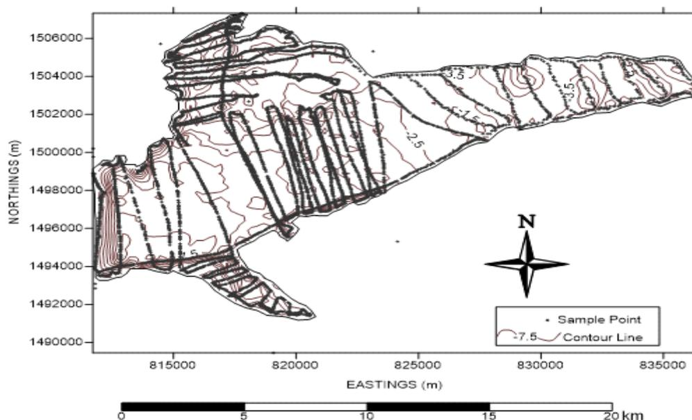
**Figure 3:** Current Bathymetric Map of Goronyo Reservoir Generated by Surfer 11
