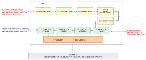
Flow diagram water supply distribution in pilot zone 2 (From water works sector 12)
