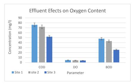
Fig. 2. Effluent effects on oxygen content
