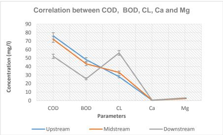
Fig 6: Correlation between COD, BOD<sub>5</sub>, Chlorine, Calcium and Magnesium concentrations
