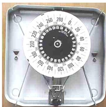
**Plate 1:** The internal part of the analogue scale
