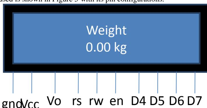
**Figure 5:** The LCD package with its pins configuration.
