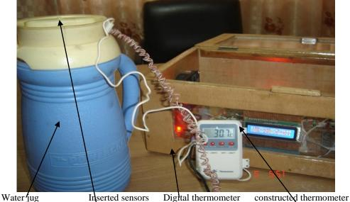
ug Inserted sensors Digital thermometer constructed thermometer Plate 4: Set up of experiment
