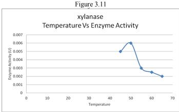
It is evident from Fig. 3.11 that xylanase enzyme from *P.chrysogenum* was exhibited its optimal activity at 50°C.
