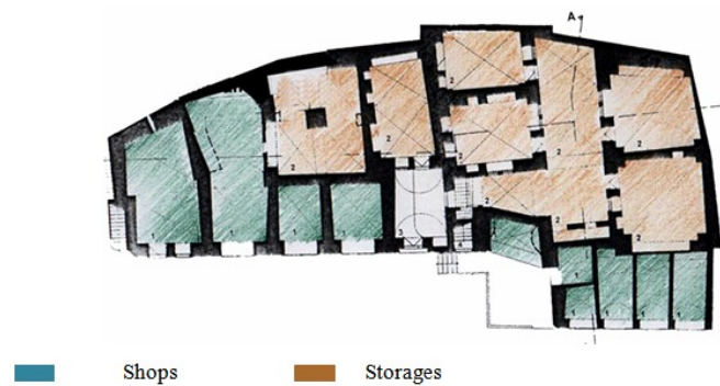
Fig. 6 Abu Jaber house basement floor multi-use plan: it accommodated both commercial and residential functions as well. Source: Author 2013
