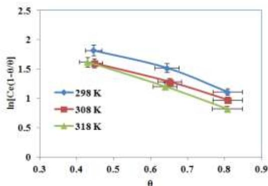
**Fig.9.** Fowler-Guggenheim adsorption isotherm plots for adsorption of MB onto PSCFS.
