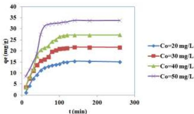
**Fig. 1.** Effect of contact time and initial dye concentration on dye removal. PSCFS dose 4 g/L (natural initial pH, at 298 K, agitation speed 150 rpm).
