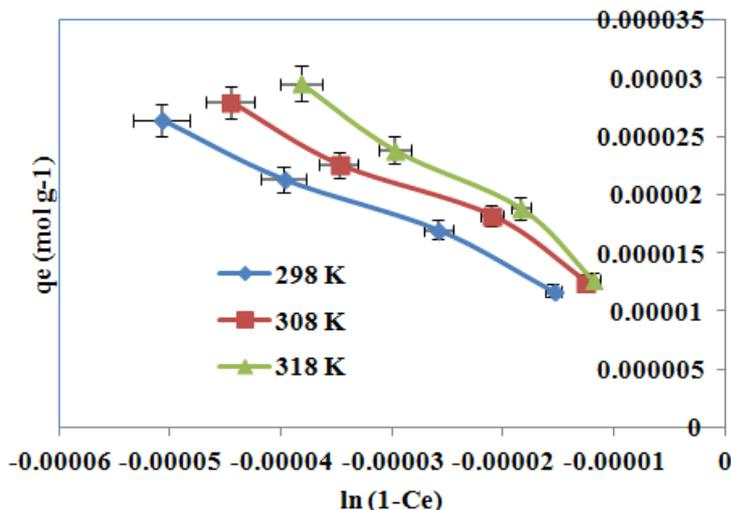
Fig.13. Smith adsorption isotherm plots for adsorption of MB onto PSCFS.
