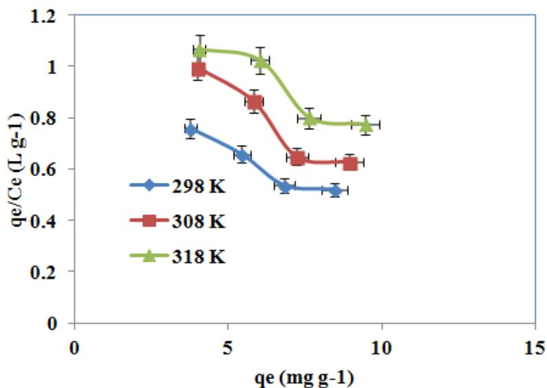
Fig.15. Scatchard adsorption isotherm plots for adsorption of MB onto PSCFS.
