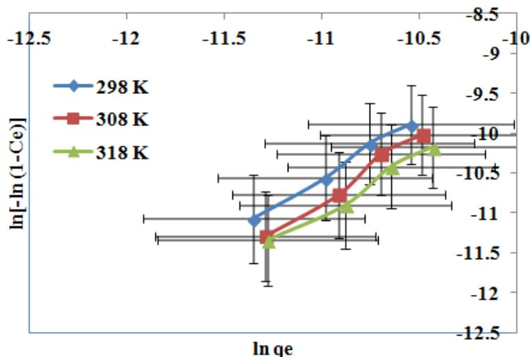
Fig.12. Henderson adsorption isotherm plots for adsorption of MB onto PSCFS.
