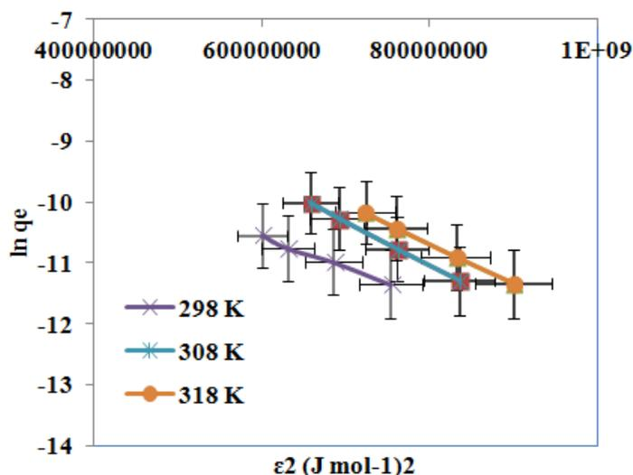
Fig.4. DKR adsorption isotherm plots for adsorption of MB onto PSCFS.
