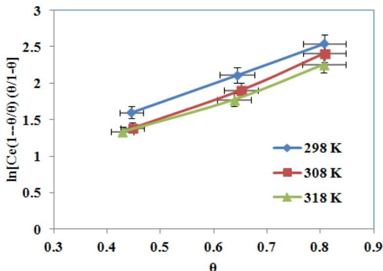
Fig.10. Frumkin adsorption isotherm plots for adsorption of Methylene Blue onto PSCFS.
