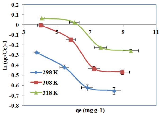
Fig.8. Elovich adsorption isotherm plots for adsorption of MB onto PSCFS.
