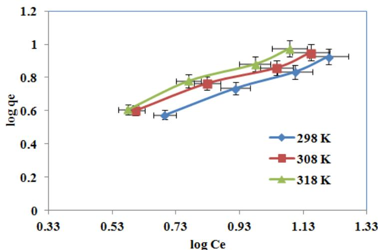
Fig.11. Halsey adsorption isotherm plots for adsorption of MB onto PSCFS.
