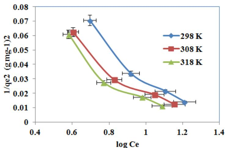
Fig.7. Harkins-Jura adsorption isotherm plots for adsorption of MB onto PSCFS.
