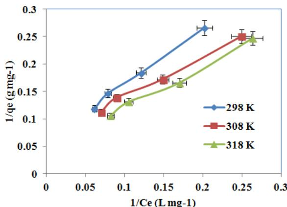
Fig.2. Langmuir plots for adsorption of MB by PSCFS.
