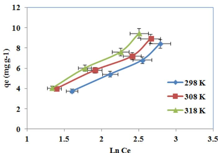
Fig.5. Temkin adsorption isotherm plots for adsorption of MB onto PSCFS.
