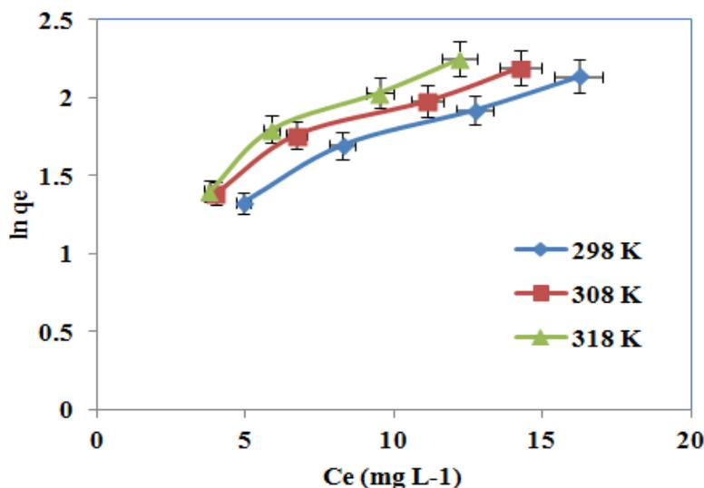
Fig.14. Jovanovic adsorption isotherm plots for adsorption of MB onto PSCFS.
