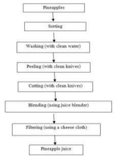
Fig 1: Unit operation for the production of pineapple juice
