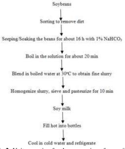
Fig 2: Unit operation for the processing of soy milk
