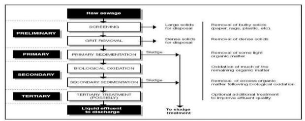
Figure 1. Typical stages in the conventional treatment of sewage
