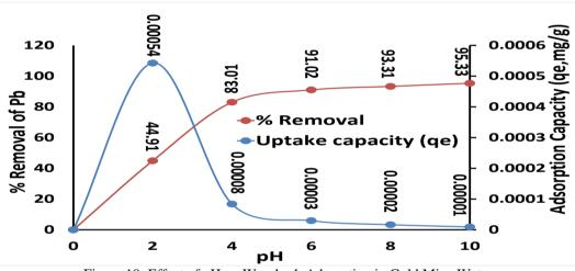
Figure 10: Effect of pH on Wood ash Adsorption in Gold Mine Water
