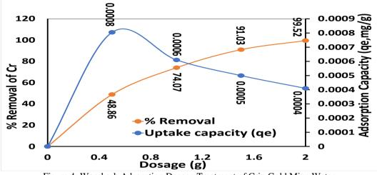
Figure 4: Wood ash Adsorption Dosage Treatment of Crin Gold Mine Water
