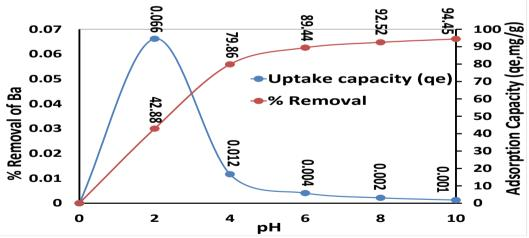
Figure 8: Effect of pH on Wood ash Adsorption of Ba in Gold Mine Water
