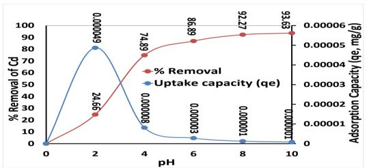
Figure 7: Effect of pH on Wood ash Adsorption of Cd in Gold Mine Water
