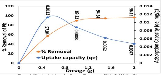
Figure 5: Wood ash Adsorption Dosage Treatment of Pbin Gold Mine Water
