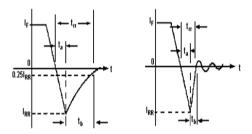
a. Soft recovery b. Abrupt recovery Fig. 3 Reverse Recovery Current Characteristic
