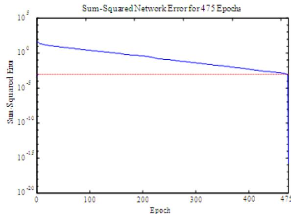
**Fig. 4** Error convergence of ANN-I (Model I) for L-L faults in training
