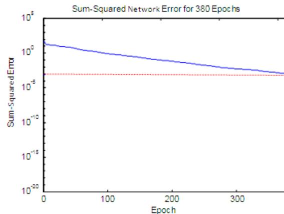
**Fig. 5** Error convergence of ANN-II (Model I) for L-L faults in training
