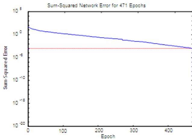
Fig. 10 Error convergence of ANN-I (Model II) for L-G faults in training
