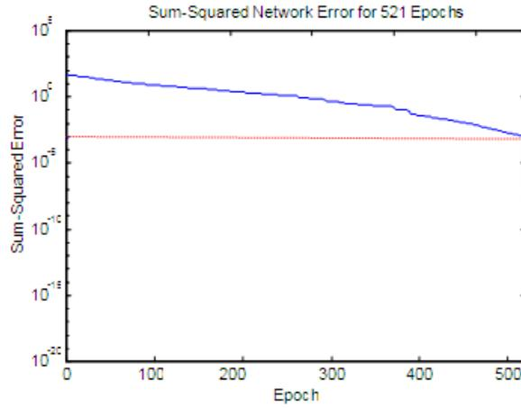
Fig. 6 Error convergence of ANN-I (Model I) for L-G faults in training
