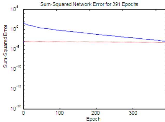
Fig. 9 Error convergence of ANN-II (Model II) for L-L faults in training
