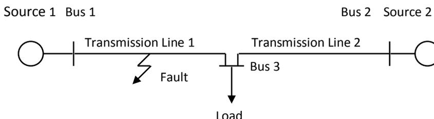
**Fig. 2: A faulted transmission line fed from both ends**
