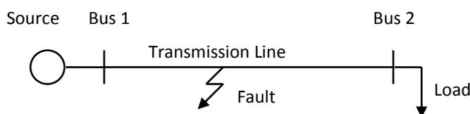
Fig. 1: A Faulted Transmission Line Fed from One End
