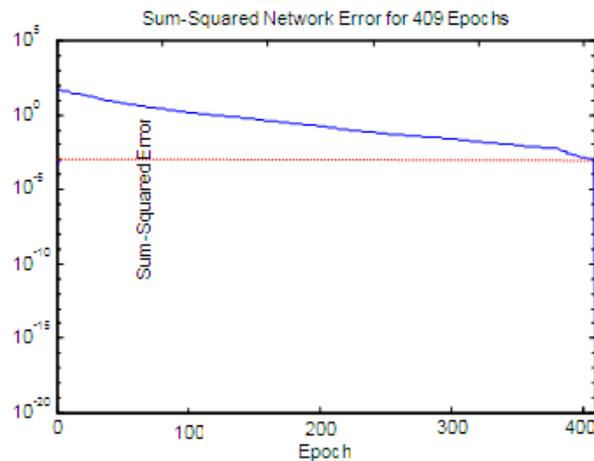
Fig. 11 Error convergence of ANN-II (Model II) for L-L faults in training
