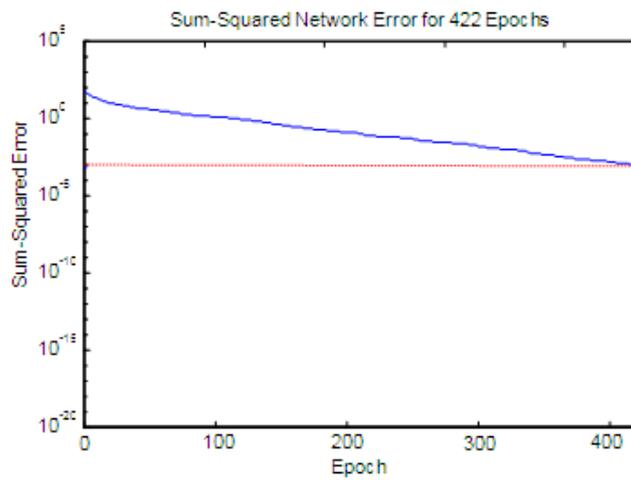
Fig. 8 Error convergence of ANN-I (Model II) for L-L faults in training
