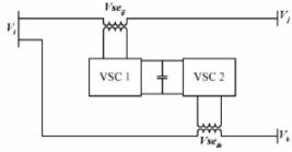
Fig: Schematic diagram of two converter IPFC
