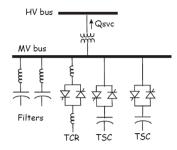
Fig: Circuit Diagram of Static VAR Compensator
