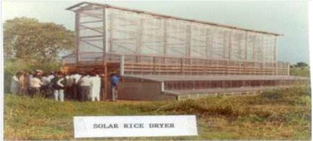
Figure 1: 2-tonne Solar Rice Dryer atAdarice Co. Enugu built by NCERD [7].
