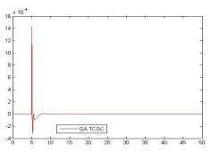
Figure2: Speed Deviation in SMIB with Fault with GA-TCSC
