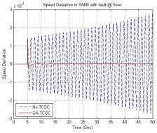
Figure3: Speed Deviation in SMIB with Fault without & with GA-TCSC
