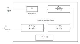
Fig.3: Block diagram of TCSC controller
