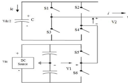
Fig.10.1.Circuit diagram of single phase multilevel inverter with capacitor
