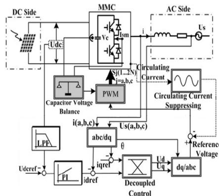
Fig.13. Modular multilevel PV inverter overall control block diagram.
