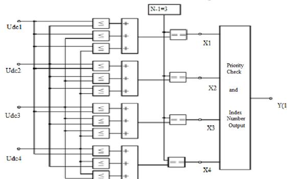
Fig. 6 (a) Index acquirement method of the MIN voltages block diagram.
