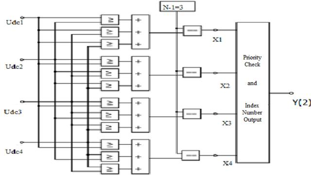
Fig.6 (b).Index acquirement method of the MAX voltages block diagram.
