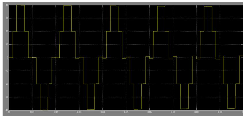
Fig. 11. single phase multilevel inverter with capacitor output voltage
