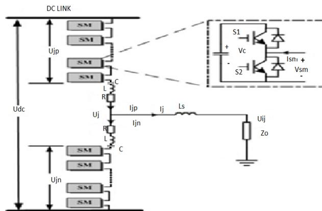
Fig.10. Single phase equivalent circuit of multilevel inverter
