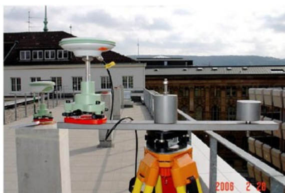
Figure 6. Rover Antenna mounted on a tripod provided with a rotating arm
