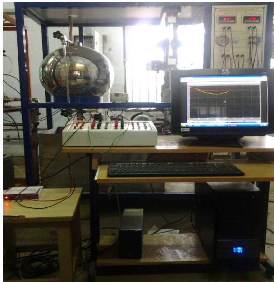
Fig 7. Closed loop apparatus setup of Spherical tank level process (Real time)
