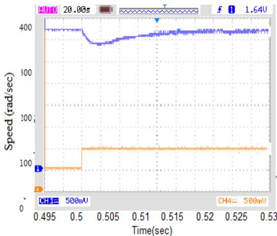
Figure 18 Virtual motor speeds when torque increases Figure 19 MATLAB speed when load torque increases
